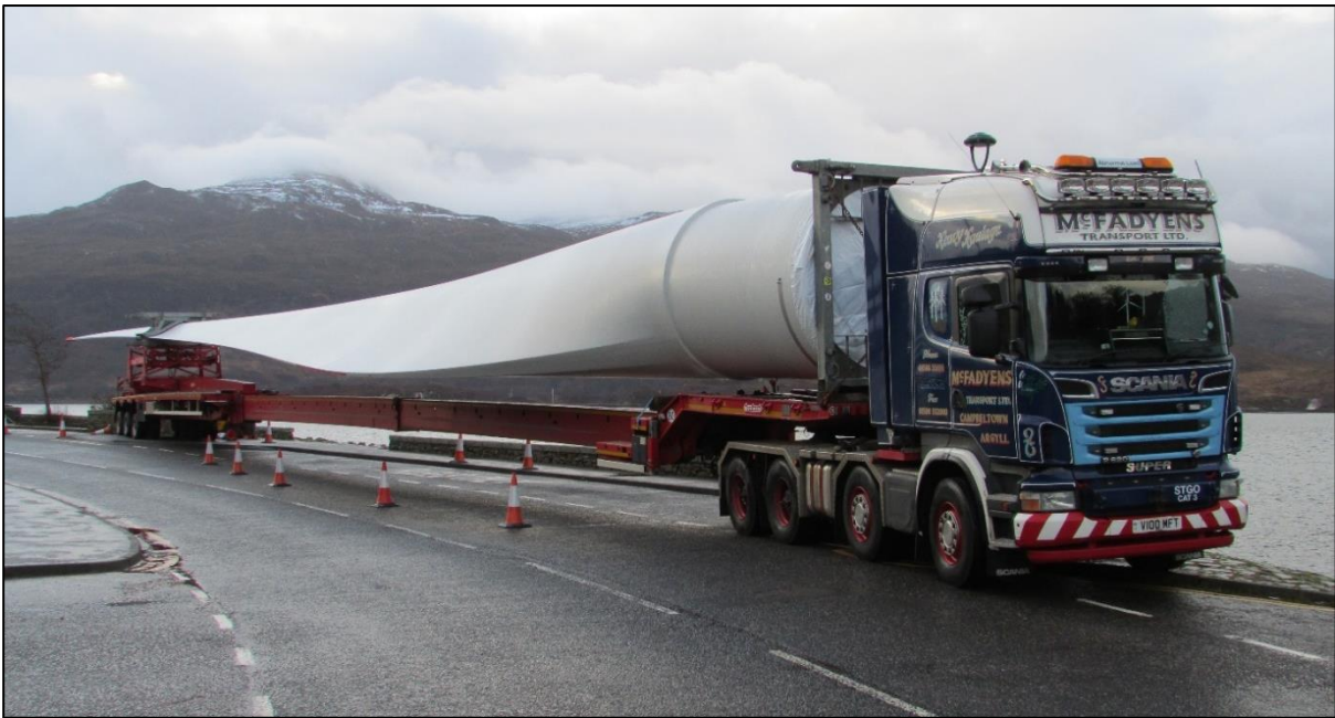
Figure 3 Super Wing Carrier with Loaded Wind Turbine Blade
