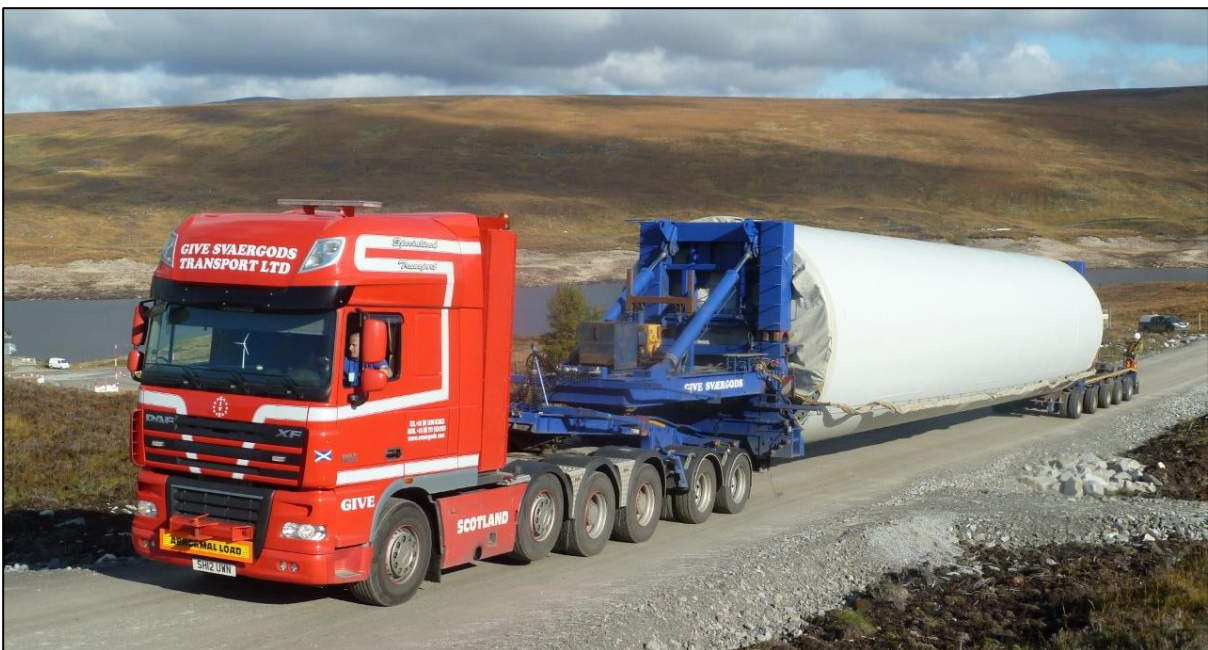
Figure 3 Super Wing Carrier with Loaded Wind Turbine Blade
